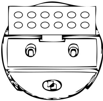
Remove adhesive film from pad and line up margins carefully, before fixing it.
