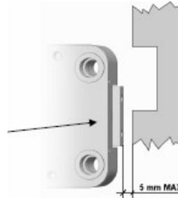
Any component that is fixed to the bolt, must be approved before use.
