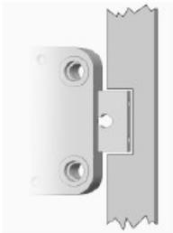
In the LOCKED position, there should be approximately 1 mm clearance between the lock bolt and the cavity in the blocking bar of the boltwork. The lock bolt must move freely into the cavity.
