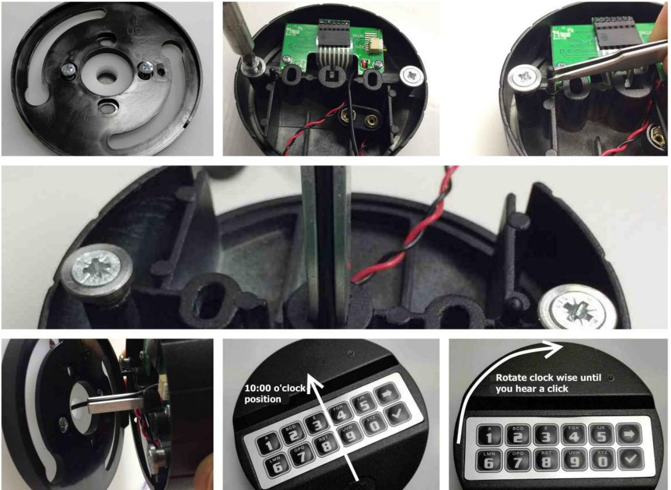
Cut the grooved shaft to the appropriate length: measure door thickness (from mounting surface of the entry unit to the mounting surface of the lock) and add **40 mm (1.6")**. Prepare the mounting and cable holes. Fix the screws (M4) / Imperial 8-32 UNC and the rotating back plate, placing it on the "UP" to permit the keypad rotation.
