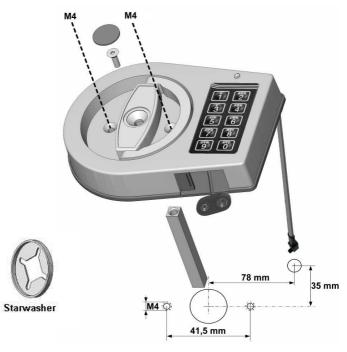
Cut the 8mm square shaft to an appropriate length. Make sure the shaft drives extends into lock or boltwork properly. Affix the shaft with the provided screw in the handle and cover the screw with the label. Route the cable through the cable hole. Push the shaft as shown above into the boltwork. Lock and boltwork must be in the "OPEN" position.
