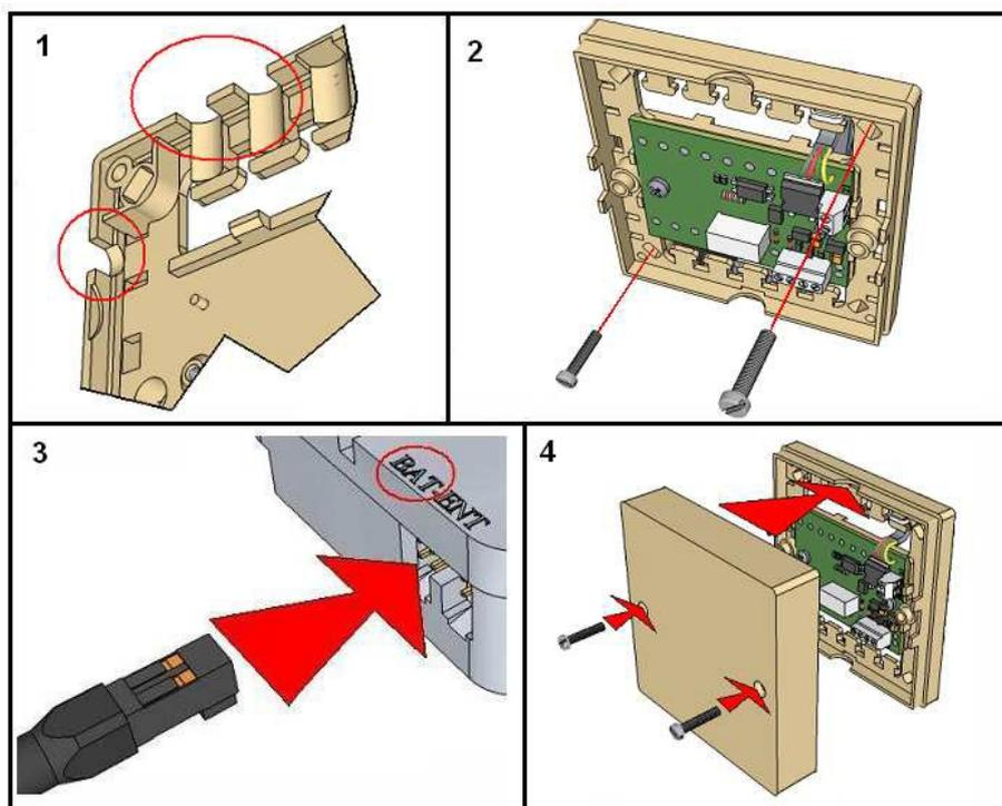
1. Cut out enough openings for the cables in the cover to be used on the underside of the base.
