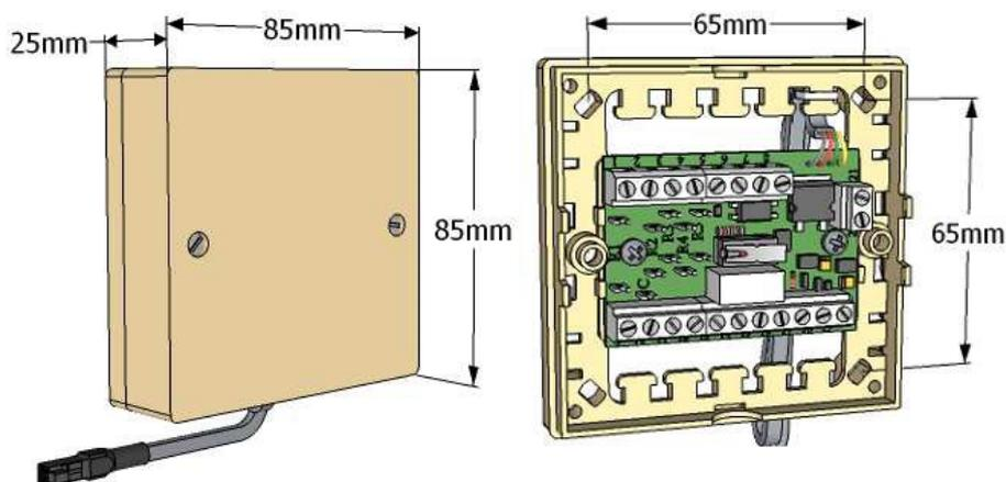
When deciding position to fit the boxes make sure that no moving part of boltwork will interfere with box or cable when in use. Cable length is approximately 350mm (usable). De-burr fixing holes (2x M3 screws min) and clean surfaces.
