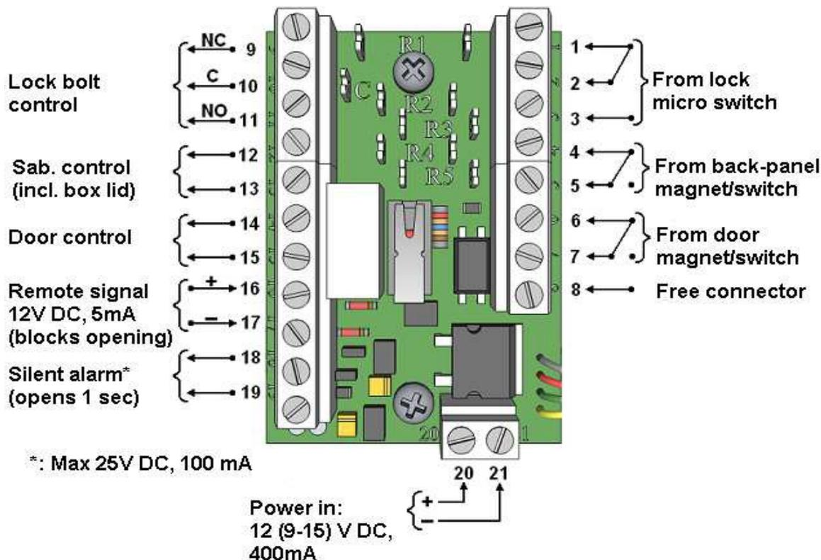
**Note: Resistor R1 to R5 are not included and must be installed on the board by yourself.**
