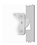
In the **LOCKED** position, there should be approximately 1 mm clearance between the lock bolt and the cavity in the blocking bar of the boltwork. The lock bolt must move freely into the cavity.
