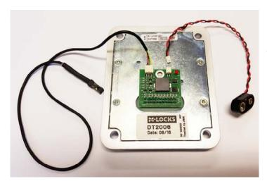
M-LOCKS recommends to fit the emergency power contact in order to ensure a quick opening of the cabinet if the inside battery ran empty.
