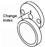
Fit escutcheon on outside of safe (if used) making sure that change index is properly aligned according to lock handing.
