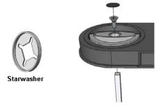
Cut the 8mm square spindle shaft to an appropriate length. It is recommended to chamfer cut end slightly for spindle to easier enter the lock/boltwork during next step. Make sure the shaft will extend properly into the lock or the boltwork. Affix the shaft with the provided screw in the handle and cover the screw with the label.
