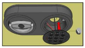
Do not remove and re-apply keypad once it has been glued in the housing!
