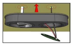
Before proceeding, make sure that the lock/boltwork is in the **open position**. Turn the pull handle so that the handle base is vertical and mounting holes are visible. Hold the unit horizontal and guide spindle shaft and keypad cable through holes and into lock/boltwork and push unit flat against mounting surface.
