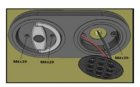
Thoroughly clean the edge where keypad foil is to be attached with Methyl ethyl ketone (MEK) MEK can be obtained p.ex. by: Bleko, Kempertec, merz+beteli ag. The area must be dry and clean for glue to catch properly. Feed the keypad cable through the cable hole. Remove the protective layer from the adhesive ring on the back of the keypad unit. Position the keypad and press it into the housing.
