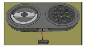
Connect one (1) battery to the battery connector. Only use 9V ALKALINE Duracell Procellor Energizer batteries.
