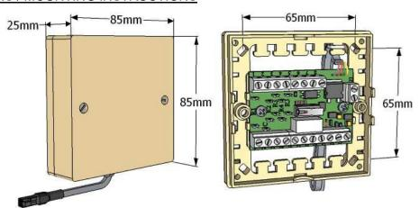
When deciding position to fit the boxes make sure that no moving part of boltwork will interfere with box or cable when in use. Cable length is approximately 350mm (usable). De-burr fixing holes (2x M3 screws min) and clean surfaces.
