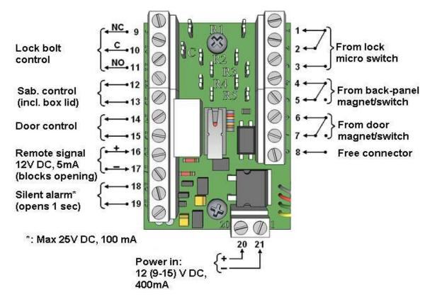
Note: Resistor R1 to R5 are not included and must be installed on the board by yourself.
