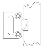
If the RevoBolt lock is used in conjunction with another lock, the boltwork must be constructed in a way that the RevoBolt secures first.
