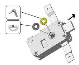
Insert the connector of the entry unit as shown in the outer position. Check that the connector is completely seated and locked by the black cable retainer. To remove the connector, use a small screwdriver to push down the cable retainer. Tie cables away from moving parts and sharp corners.
