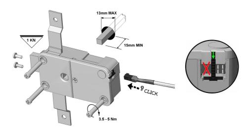
For unplugging the connector lock has to be depressed. Connect a 9V alkaline Duracell , Energizer or Duracell Industrial- battery to the battery clip to the keyboard ( or battery box ), and check the lock functions. Keep the Cable from sharp edges or moving Boltwork parts and set permanently.
