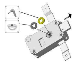
Insert the connector of the entry unit as shown in the outer position. Check that the connector is completely seated and locked by the black cable retainer. To remove the connector, use a small screwdriver to push down the cable retainer. Tie cables away from moving parts and sharp corners.
