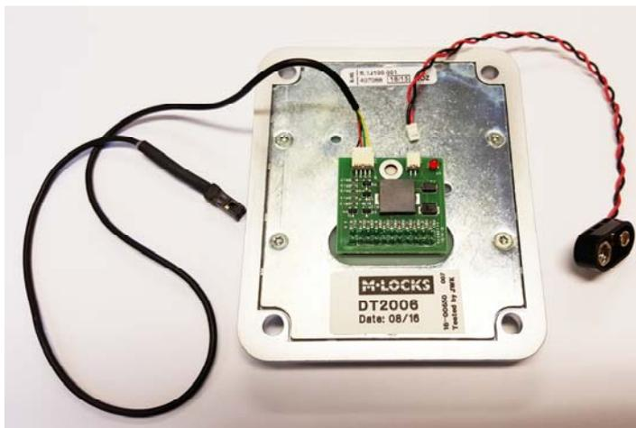
M-LOCKS recommends to fit the emergency power contact in order to ensure a quick opening of the cabinet if the inside battery ran empty.
