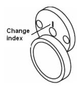
Insert the change key into the change key hole at the back of the lock (inside the door). Turn the key about 90° to the RIGHT until it stops. Turn the operating key / setup key to the left and take it out.
