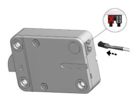
Insert the connector of the entru unit in the outer (ENT) position. Connect battery / alarm box connector (if used) in the inner (BAT) position. Check that the connector(s) is completely seated.
