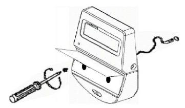
Remove the protective film from the membrane, carefully align the margins and stick it to the housing.
