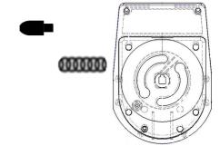
Insert the spring and the pin into the hole on the back cover.
