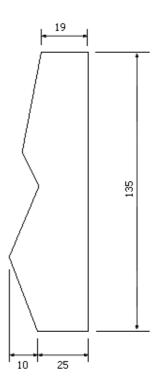
With mounting plate add 3mm to thickness; with turnable plate add 9,7mm.
