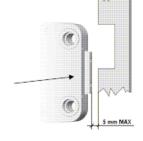
The force applied to the bolt must not exceed 1kN.
