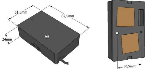
When positioning the boxes make sure that no moving part of boltwork will interfere with the box or cable when in use. Cable length is approximately 400mm (usable). Prepare cut-out and fixing holes and clean the surfaces.
