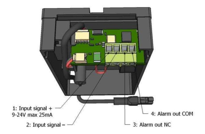
Never use excessive force when tightening the screw connectors. Try all functions several times after box has been connected. Use only Duracell or Energizer ALKALINE 9V batteries.
