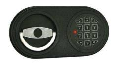
The EuroLine series was specially developed for safes using boltworks where the C/C measurement between lock and boltwork drive is 100mm. It will also work combined with the EM1620 (EM1520) DirectDrive lock. The ABS housing of the EuroLine Entry unit combines an alpha-numeric foil keypad with a pull handle (metal) and an integrated battery compartment. The 8x8 mm square shaft of the pull handle drives either the lock or a boltwork. Cable length is approximately 30 cm.
