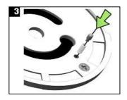
Insert first the spring and then the pin into the hole on the back cover
