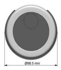
The terminal for the electronic key (Dallas Key) and or communication is located on the front next to the LED. In case this terminal is not required, it should be covered with the provided round black label.
