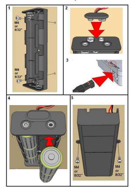
Fit housing using 2x M4 or 8/32" screws (1). Route and connect cable to box (3) and BAT connection on lock (4). Note that picture is for illustration only, BAT connection can be placed differently dependant on lock used. Tie up loose cable in a professional way. Fit six 1,5V, C-cell, brand name, ALKALINE batteries in housing observing polarity (5). Snap lid in place and fix to surface with 2x M4 or 8/32" pan-head screws (4).
