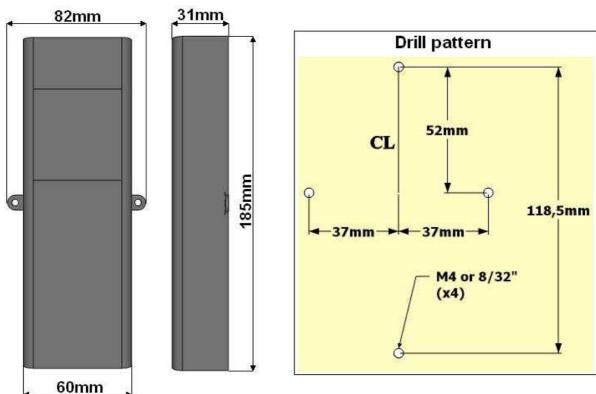
When deciding position to fit the 4001 make sure that no moving part of boltwork will interfere with box or cable when in use. Cable length is approximately 400mm (usable). Prepare fixing holes and clean surfaces.
